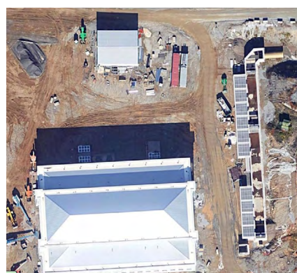
Fig 6 – Overhead view of the Bellwood Quarry pumping station under construction. The concrete flow control channel (at right above) was cast in place with Xypex Admix C-500 as part of the 5,000 psi mix. Xypex Admix provides integral waterproofing and protection that will help the structure meet its 100-year design goal.
